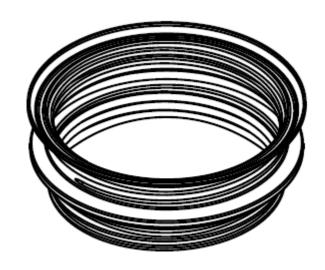
The STAR-24R6 is a threaded 6 inch riser that is designed to mate directly to the manway(s) of the Roth RMT tank, add to an existing Roth STAR-24R6 or R12 riser to meet elevation requirements. The STAR-24R6 is also compatible with the STAR-24 HPV hanging pump vault and the STAR-24DB11 distribution box.
