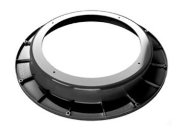
The Orenco Tank Adapter is specifically designed to fit the Roth RMT tank to facilitate the mounting of a pipe riser to the RMT tank. It is compatible with 24 in UltraRib PVC pipe. STEP system configurations that include the Orenco Biotube® vault require the use of the OR-ADP adapter for proper mounting and support of the vault.
